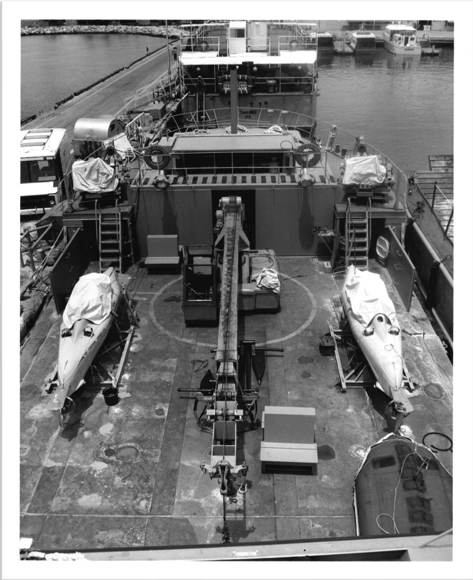
Figure 3. Perry 2-man submarines used in reentry vehicle recovery operations. Army photograph.
